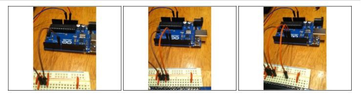
Now we will start connecting the Arduino to the display. Connect pin 4 of the display to pin 7 on the Arduino; pin 6 to pin 8; pin 11 to 9; 12 to 10; 13 to 11; and pin 14 on the display to pin 12 on the Arduino.
